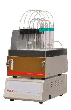
It can determine the oxidative stability of oils and fats quickly, accurately and intuitively. It is used by related departments and enterprises to study the processing, use, storage, oil selection of foods and oils, and the use of antioxidants and synergists. The oxidative stability study of methyl ester FAME and the like provides an effective scientific basis.
